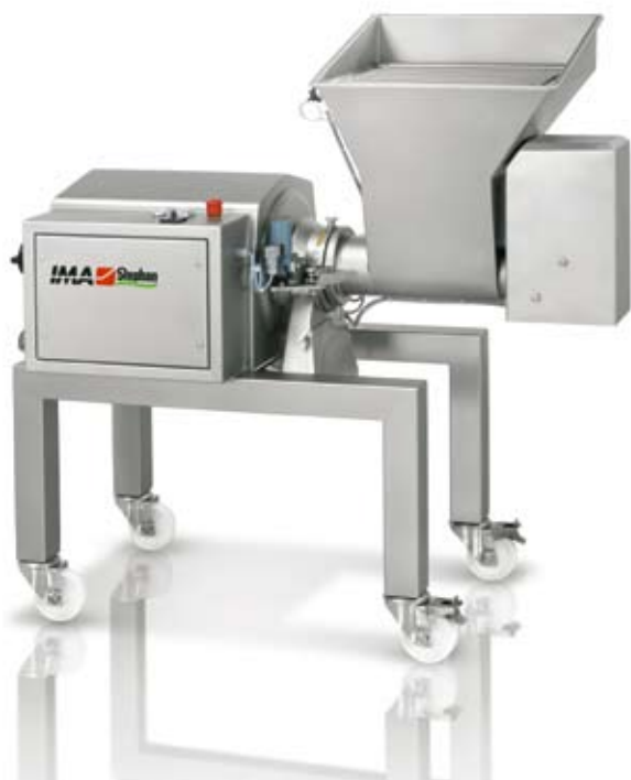
STEPHAN MCH-20K / MCH-150K GRINDING OF DRY/FROZEN PRODUCTS
